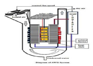
Fig. 4: AWG with Peltier effect powered by Solar energy.
