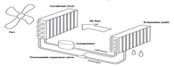
Fig. 1: Dehumidification by Refrigeration
