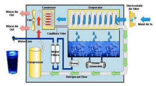
Fig. 2: Conventional Atmospheric Water Generator
