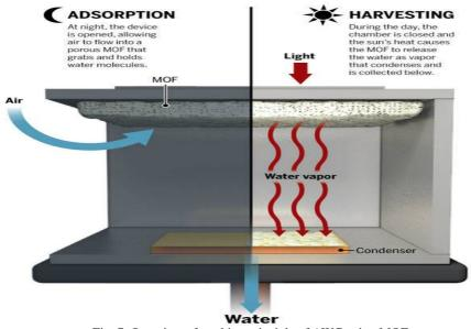
Fig. 7: Overview of working principle of AWG using MOFs.
